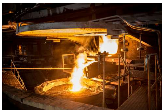
Pouring liquid metal from an arc furnace
